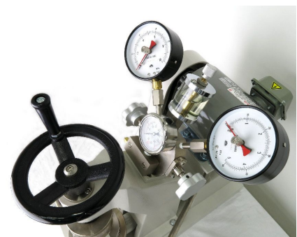
Pressure gauges indicate even pressure loads for each test
