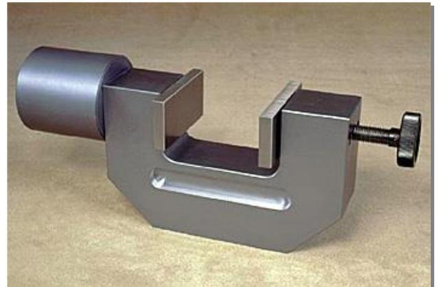
**Applications** Pneumatic grips use air pressure to actuate cylinders to provide constant clamp loads to test specimens of a wide variety. They are best suited to the following mechanical testing needs:
