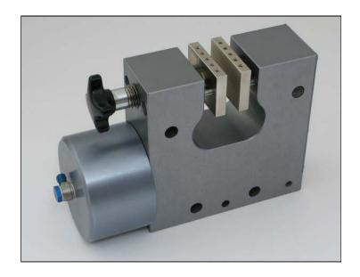
These universal grips feature an air operated clamping piston that closes one jaw via an internal lever arm with adjustments for three different sample thickness ranges. The air operated jaw then closes against a manually adjustable face jaw. The grips feature several save sample loading time with quick and easy specimen insertion.
