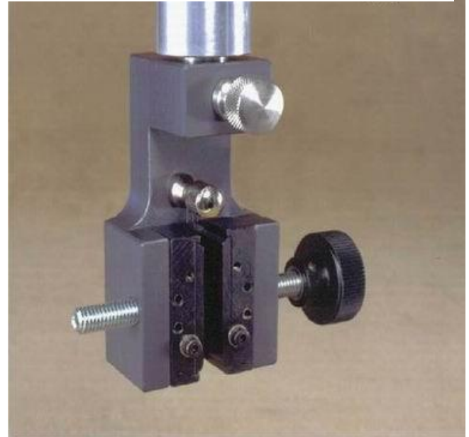
G9 Special Wire Grips for fragile small wire samples
