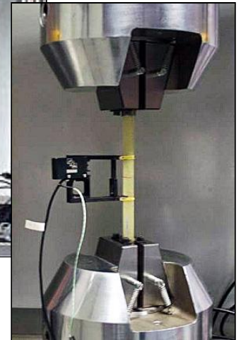
Glass fiber composites are a common test application where hydraulic clamping and wedge action is important.
