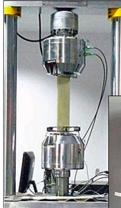
Glass fiber composites are a common test application where hydraulic clamping and wedge action is important.
