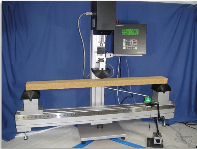
GD1037 3 Point Bend Test Fixture set up with 100P Family Universal Test Machine and E3540 Deflectometer
