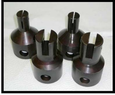
**Reference:** ASTM Standard D2095, 2008, "ASTM D2095 Standard Test Method for Tensile Strength of Adhesives by Means of Bar and Rod Specimens," ASTM International, West Conshohocken, PA, 2007, www.astm.org.
