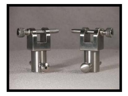
G353 Test Fixtures are made to ASTM requirements
