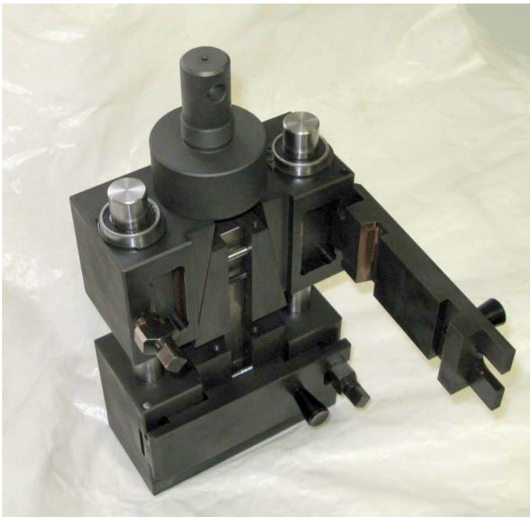
GD3410 Test Fixtures are made to exact ASTM requirements
