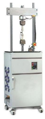
Eight digital input and eight output channels provide drive and device control. Test data can be acquired at speeds up to 5000 samples per second on all feedback channels concurrently.
